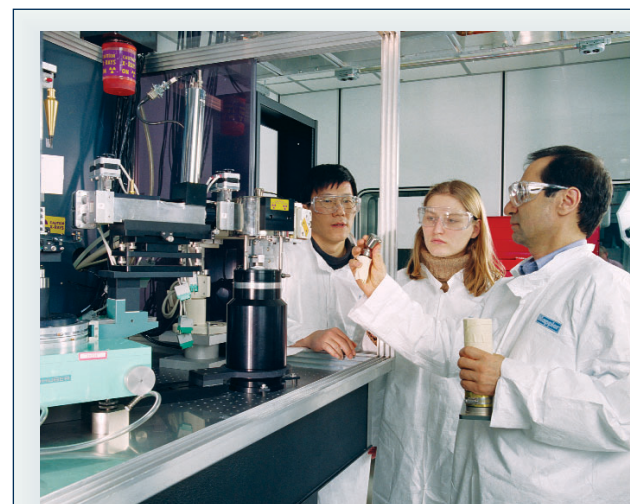
Ali Khounsary (right) , with graduate students Kristina Young and Yaming Li with the x-ray reflectometer for multilayer reflectivity measurements.
