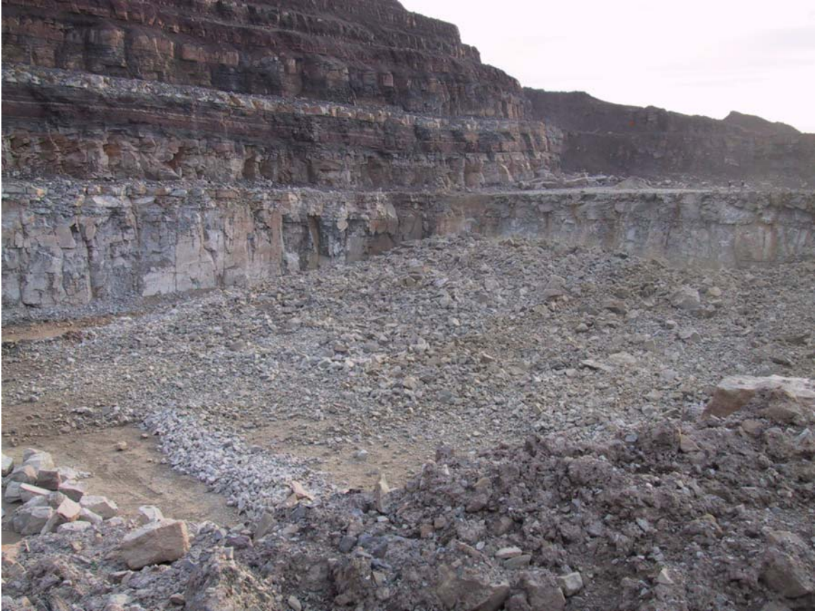
Figure 11 – Area of blasted limestone using the Daveytronic® electronic blasting system
