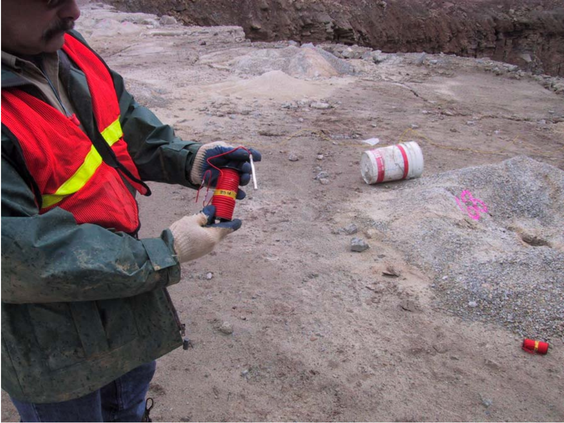
Figure 8 - Daveytronic® electronic detonator & leg wire assembly
