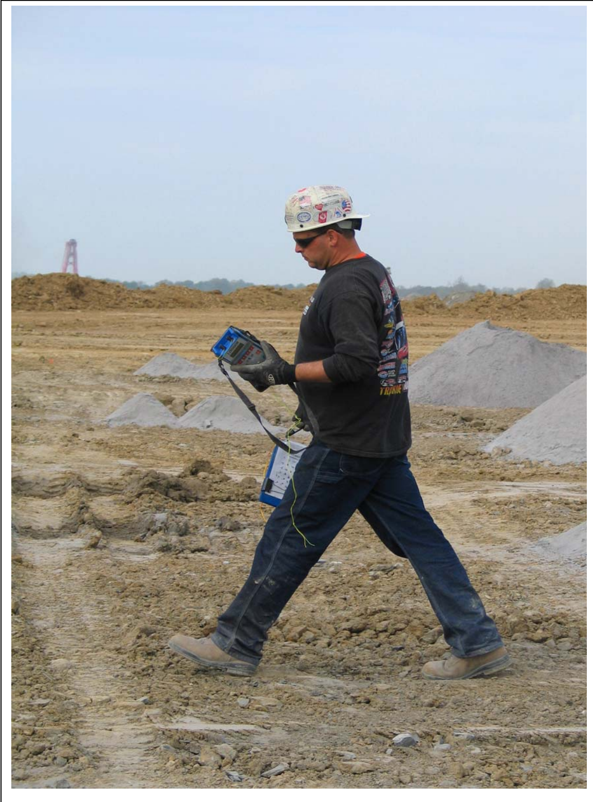
Figure 14 - Orica I-KON™ Logger used to program each electronic detonator
