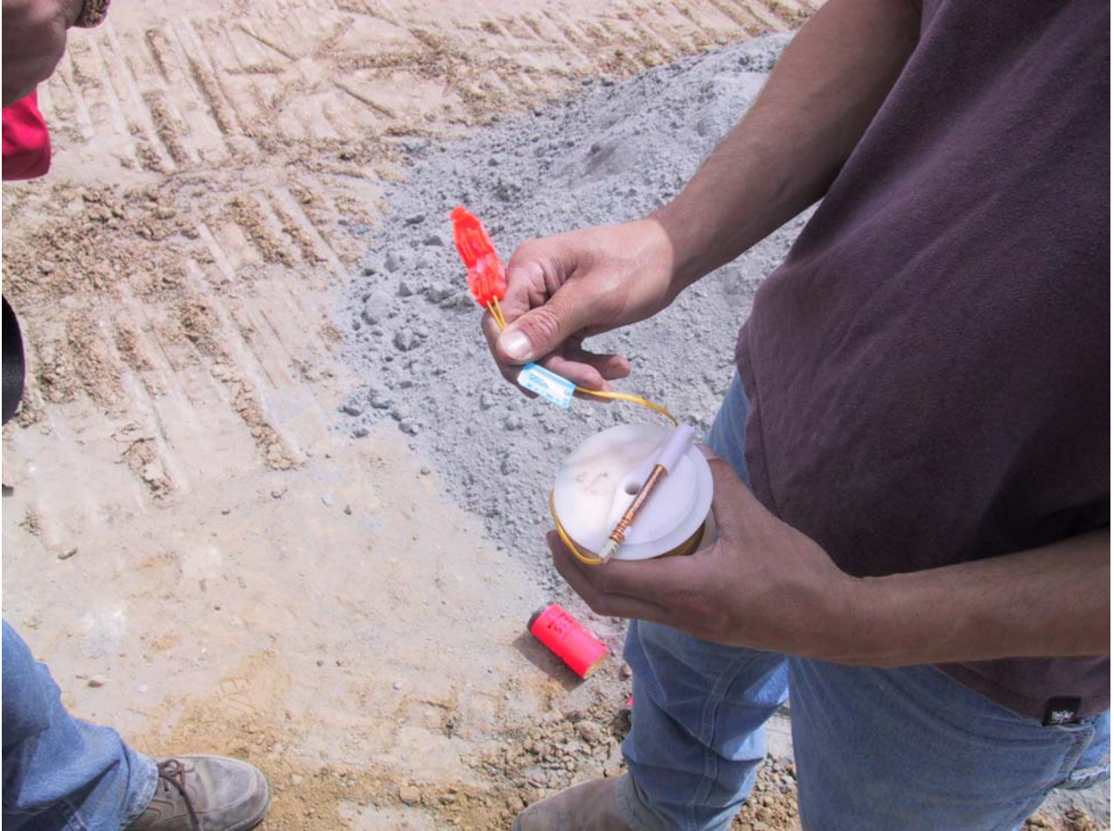
Figure 17 - Orica snap-type connector for I-KON™ electronic detonator trunk line connection
