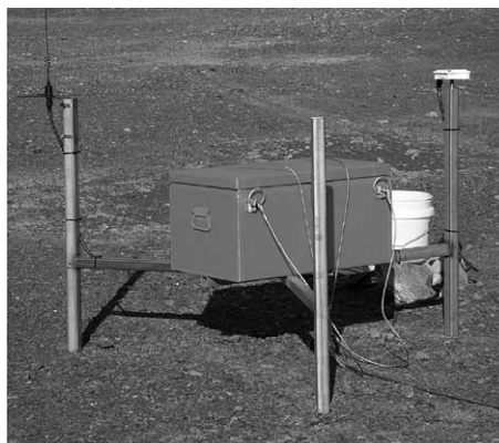
Fig. 3. Telemetered, single-frequency GPS unit used during the 2004–2005 eruption of Mount St. Helens. Each unit was slung by helicopter to its site. Over a dozen of these instruments were deployed in the crater of the volcano in 2004 and early 2005, providing valuable near-field displacement data while minimizing the hazard to field personnel.
