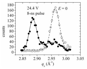
Transient strain of 2.7% in a 40 nm-thick PZT film in response to an 8 ns electric field pulse, Grigoryev *et al.* Phys. Rev. Lett. **100**, 027604 (2008).
