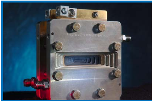
Figure 4: Cell for in situ X-ray absorption studies of fuel cell catalysts. Standard Fuel Cell Technologies cell hardware was machined to allow X-ray fluorescence studies of cathode electro-catalysts in an operating membrane-electrode assembly (fuel cell).
