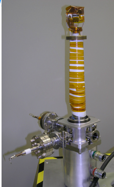
Pulsed magnetic-field up to 60T with 30 ms width for time-resolved exp
