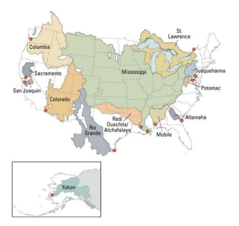
Flow, concentrations, and loads are measured at 13 sites discharging to coastal waters of the U.S. (above). Flow, concentrations, and loads are measured in 19 priority sub-basins within the Mississippi River Basin that contribute significantly to adverse conditions in the Gulf of Mexico (below).
