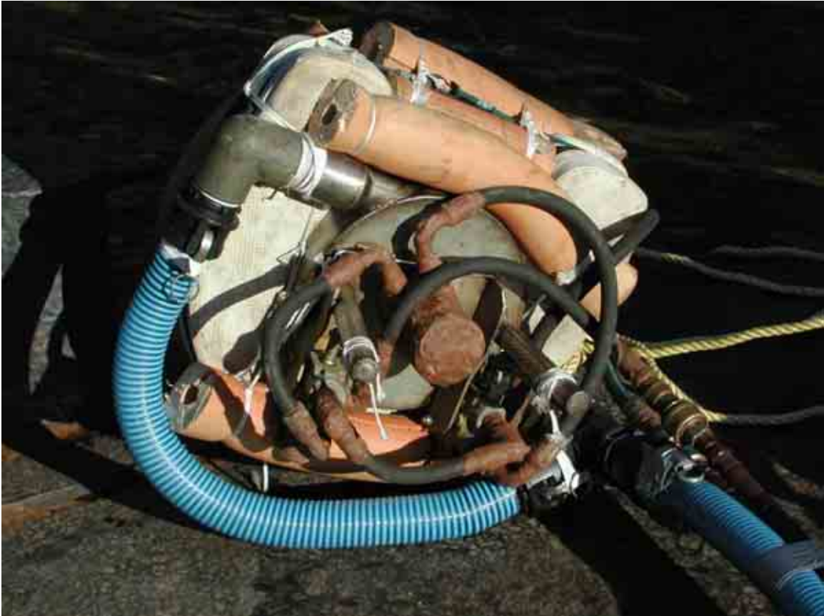
P6. The final hose configuration on the cutter with two outlets.
