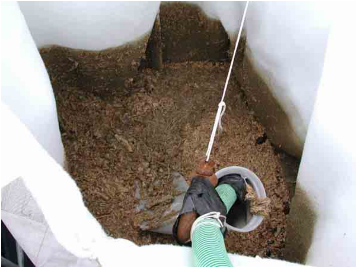
P8. First stage filter bag partially full.
