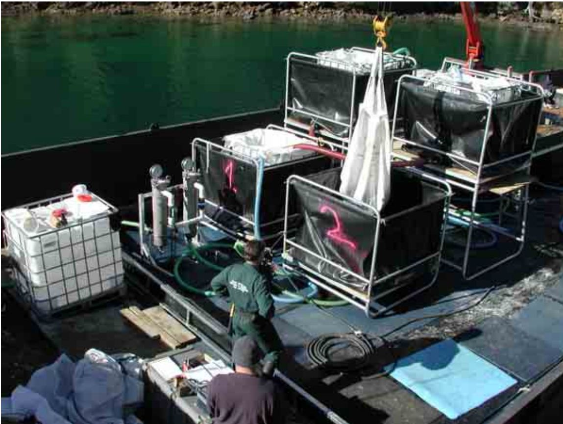
P7. Filter system on work barge “Waimarie 1”.
