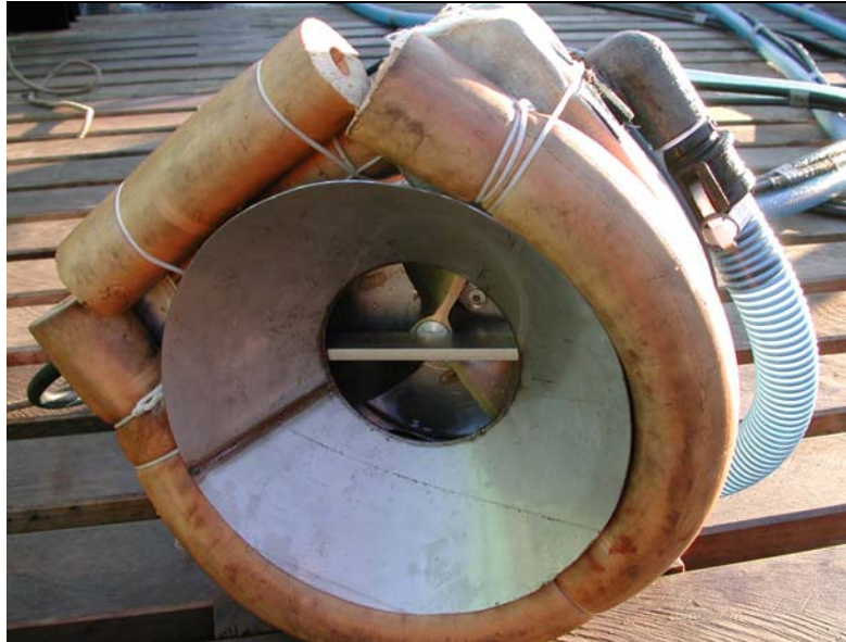
Figure 1. The original vacuum cutting head used to remove the D. vexillum from the 'Steel Mariner'. Photo courtesy of New Zealand Diving and Salvage Ltd.
