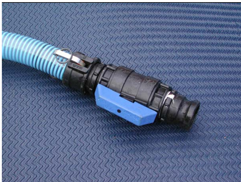
Figure 2. The diver-operated nozzle used to vacuum the D. vexillum colonies from the 'Steel Mariner' and the seabed below. Photo courtesy of New Zealand Diving and Salvage Ltd.
