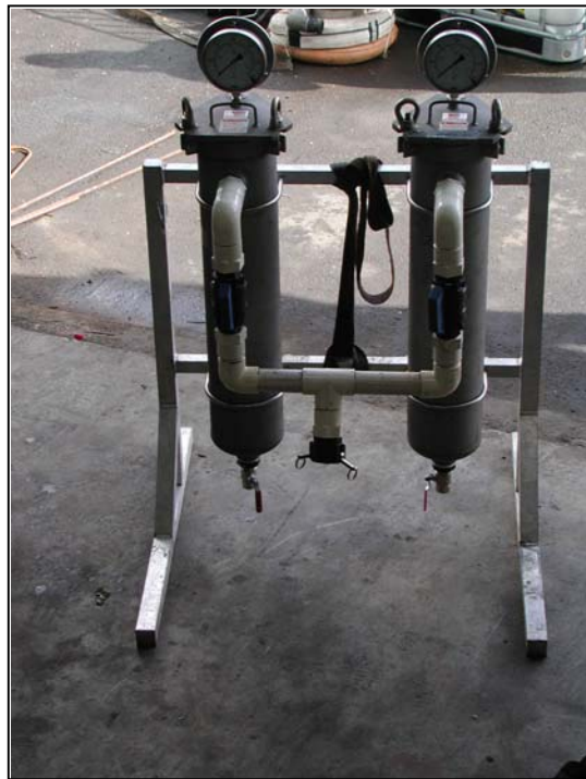
Figure 7. The effluent from Stage 2 was pumped into the BFNP bag filter vessel where 200, 100, 50, 25, 10, 5, BOS5 and 1 \mu\text{m} filter sizes were tested. Photo courtesy of New Zealand Diving and Salvage Ltd.
