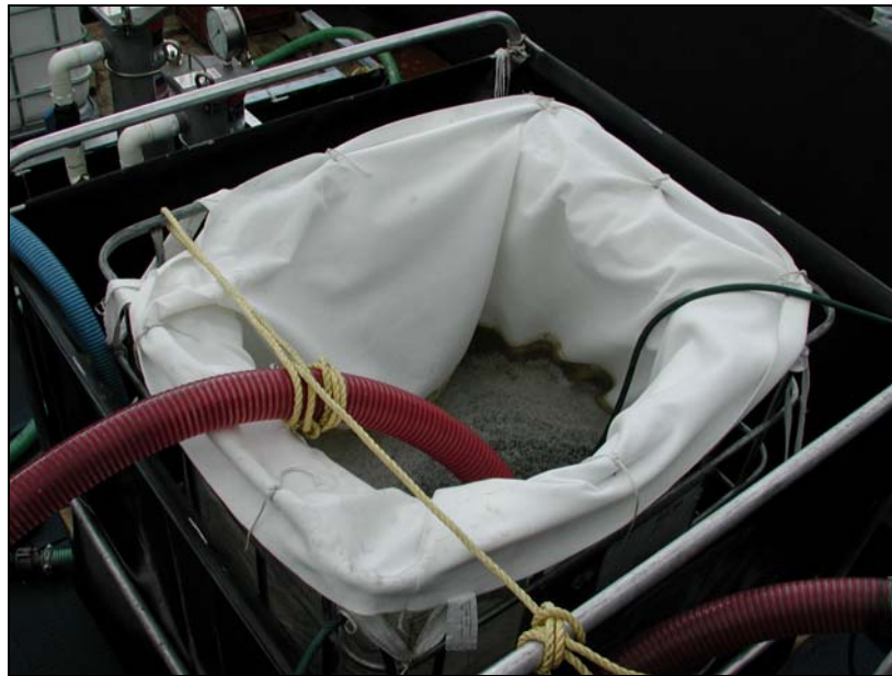
Figure 6. The effluent from Stage 1 gravity fed into Stage 2 where 200 and 100 \mu\text{m} filter liners were tested. Photo courtesy of New Zealand Diving and Salvage Ltd.
