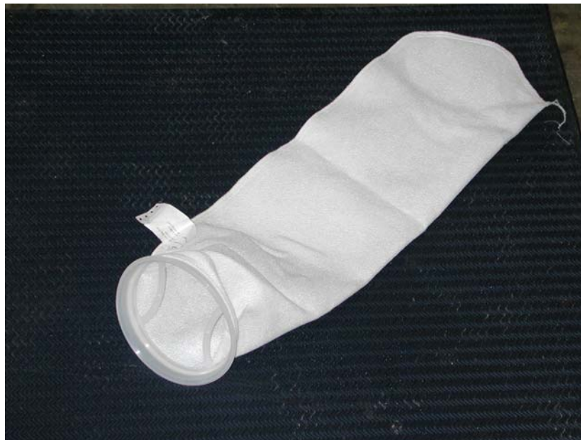
Figure 8. During Stage 3 of the filtering process 200, 100, 50, 25, 10, 5, BOS5 and 1 \mu\text{m} filter bags were tested inside the BFNP bag filter vessel. Photo courtesy of New Zealand Diving and Salvage Ltd.
