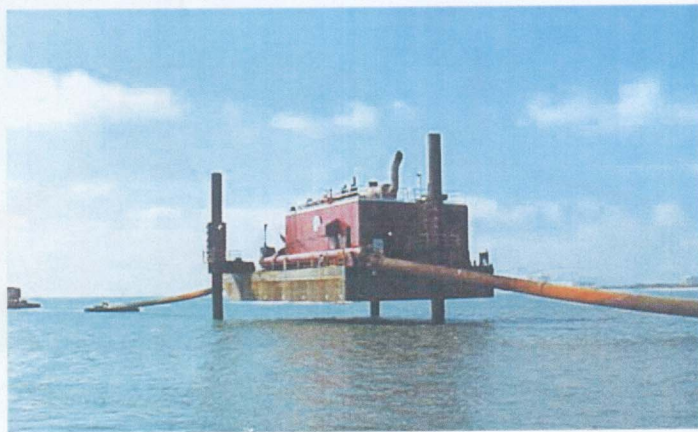
Jack-Up Booster No. 1 is raised out of the water to clear storm wave conditions.
