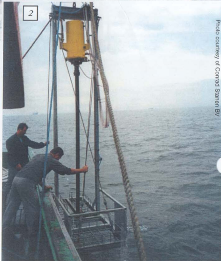
Drilling Rigs: 1) Vibrocooler with no sample tube lying horizontally on a dock. Note that the leg beneath the coiler is hinged, allowing the frame to be folded as shown for removal and attachment of sample tubes. 2) Vibro coiler with a 3-m-long barrel as it is deployed from a fishing vessel. 3) A lightweight offshore cone penetration test unit being retrieved. 4) A typical mobile light percussion drilling set-up.
