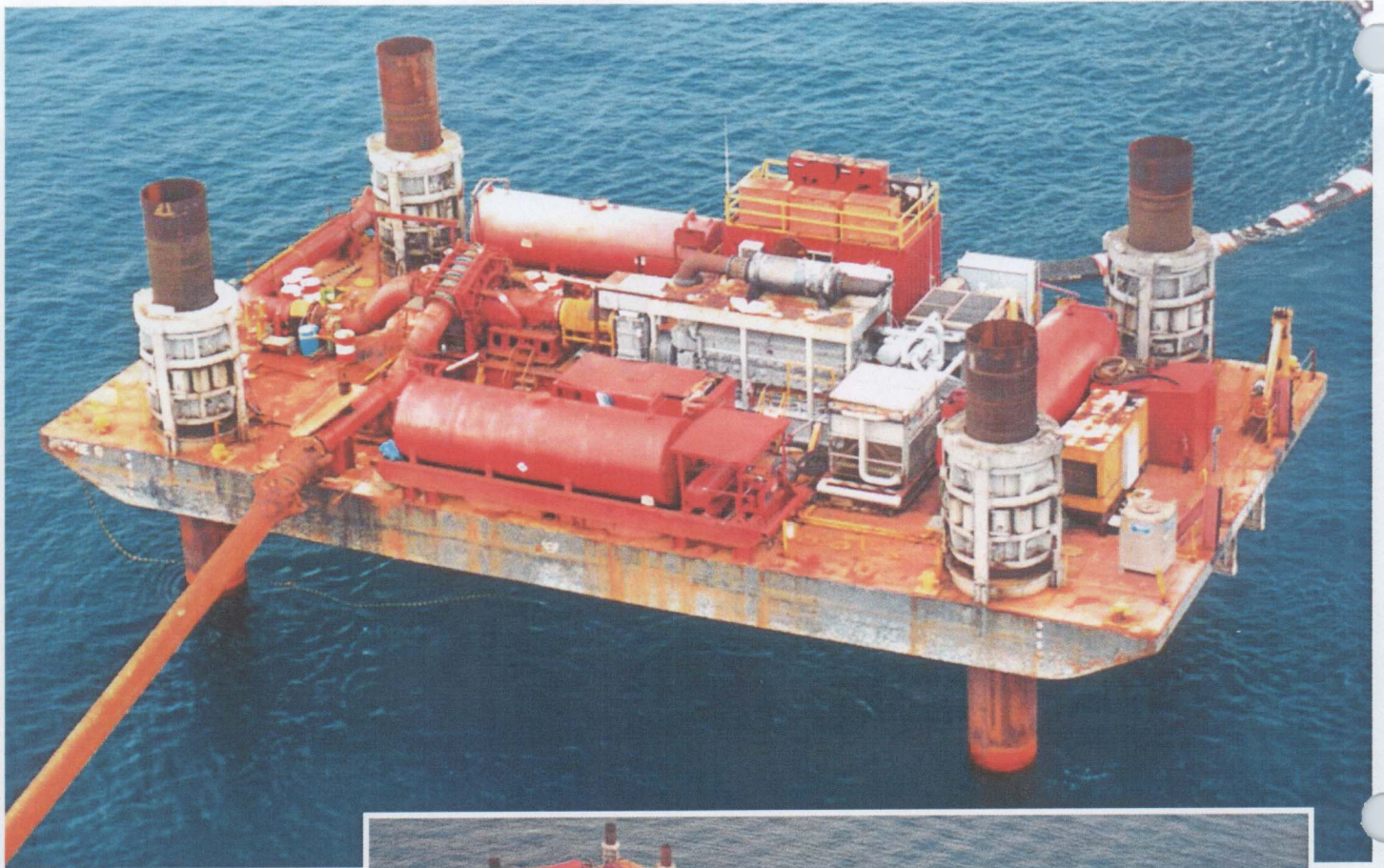
Booster No. 4 pumps sand ashore at Ft. Lauderdale, assisting the trailing suction hopper dredge Dodge Island in renovating the beach.
