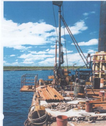
Variety of Tools & Methods: A rotary drilling rig and small cantilevered working platform are set up on a jack-up barge (above left). Test deployment of seismic reflection toufish is shown at right.
