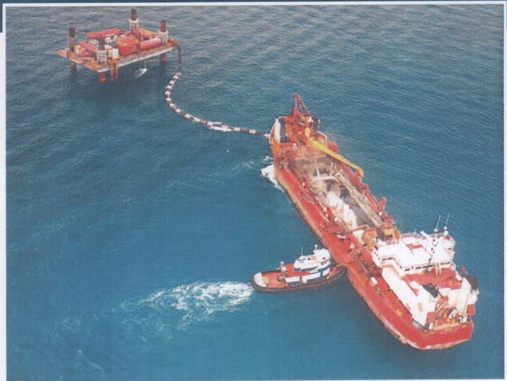
Booster No. 4 pumps sand ashore at Ft. Lauderdale, assisting the trailing suction hopper dredge Dodge Island in renovating the beach.
