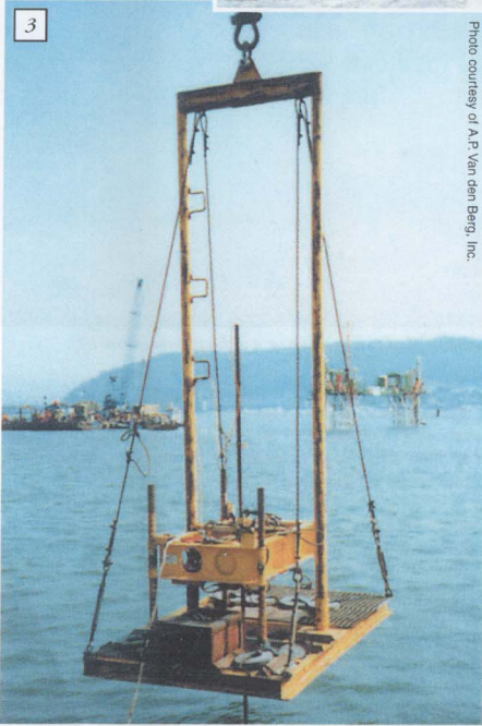
Drilling Rigs: 1) Vibrocooler with no sample tube lying horizontally on a dock. Note that the leg beneath the coiler is hinged, allowing the frame to be folded as shown for removal and attachment of sample tubes. 2) Vibro coiler with a 3-m-long barrel as it is deployed from a fishing vessel. 3) A lightweight offshore cone penetration test unit being retrieved. 4) A typical mobile light percussion drilling set-up.
