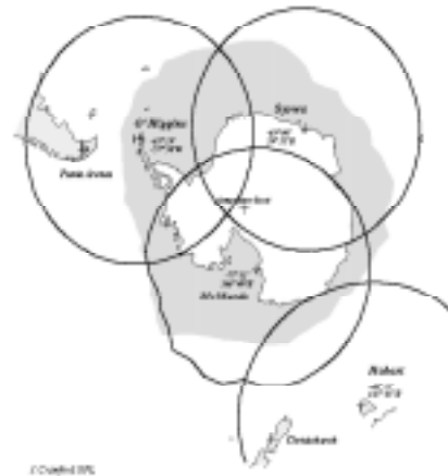
Figure 3. The nominal reception limit of NASA's McMurdo station is shown for three international SAR satellites. The other 3 ground stations are operated by Germany (O'Higgins), Japan (Syowa), and Australia (Hobart).
