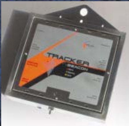
Beacon - receives and processes signal from tags
