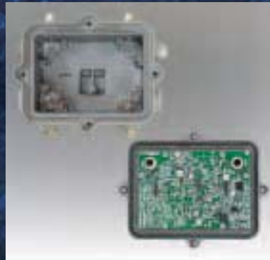
Internal casing and electronics of VDV Line Amplifier
