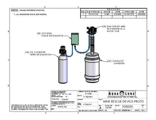
Exhibit A. Drawing of Aqua Lung Prototype Mine Rescue Device part # 105000.
