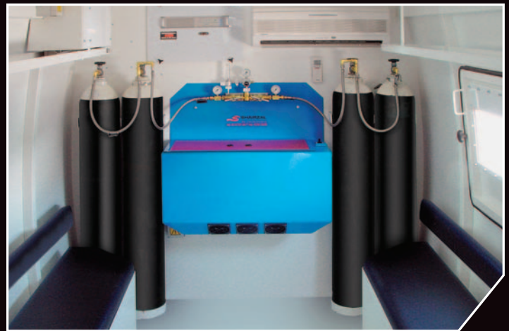
Air Scrubber Co 2 Removal
