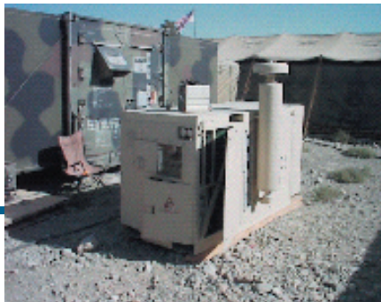
EDOCS-120 unit making medical grade oxygen for U.S. Army Combat Support Hospitals at Bagram, Afghanistan
