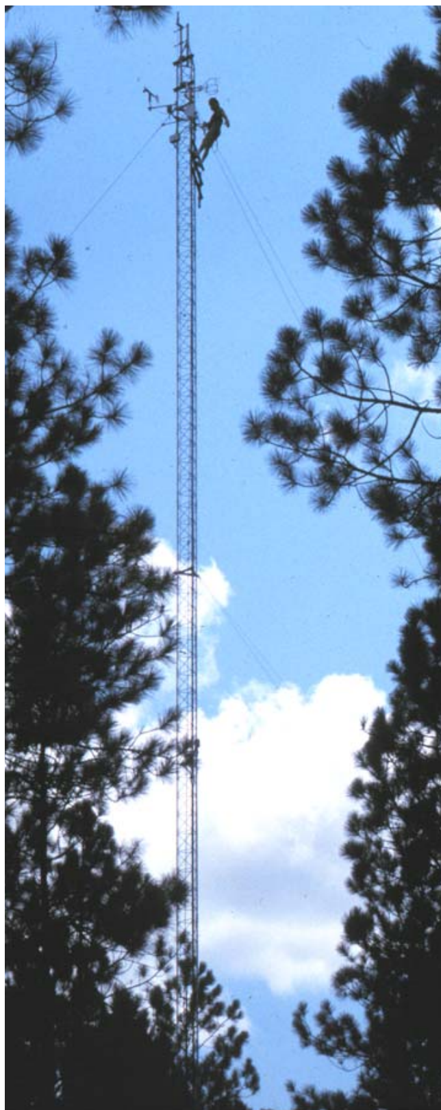
Figure 13. U.S. Geological Survey employee servicing equipment on a tower in Volusia County, Florida, used to measure evapotranspiration (ET) from an area of pine forest.
