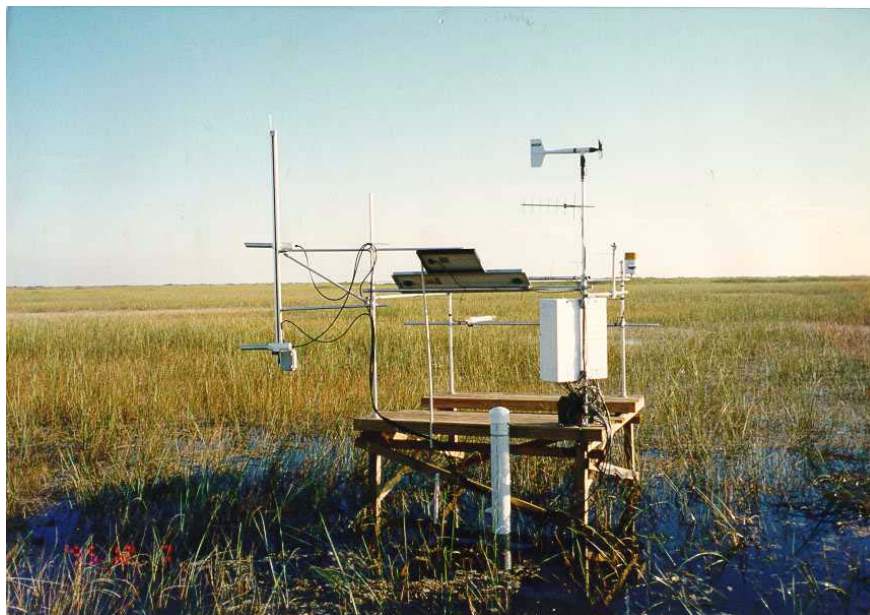
Figure 35. Sensors used for estimation of evapotranspiration using the Bowen-ratio technique in Everglades National Park.
