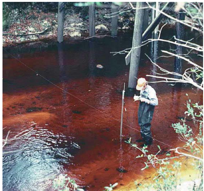
Figure 15. U.S. Geological Survey employee making a discharge measurement in a stream with tannic water.
