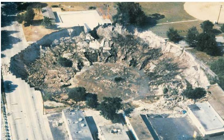
Figure 32. Aerial photograph of a large sinkhole which formed in Winter Park, Florida, May 1981.
