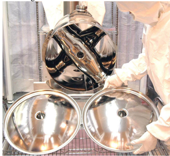
Fig. III-1. Niobium elements of the \beta 0.63 , 345 MHz, triple-spoke cavity after electropolishing, just prior to the final, closure EB welds.
