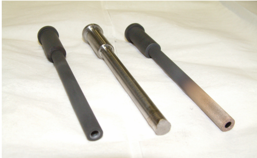
Fig. II-3. The crucibles used for titanium production. The left crucible is graphite with natural titanium absorbed into the inner wall. The middle crucible is tungsten showing the effects of the reaction at high temperature due to the nickel contamination. The right crucible is the graphite crucible used for the Ti-50 run. The silvered appearance of the graphite is still not fully explained, but is probably due to the crucible’s extended exposure to very high temperatures.
