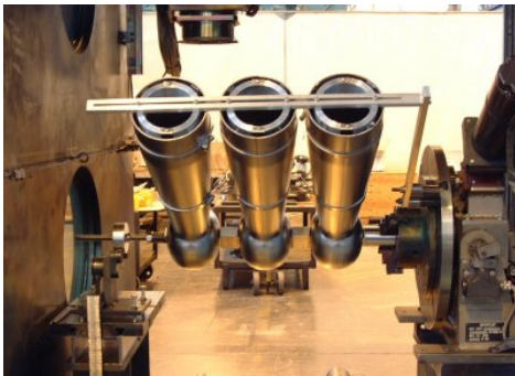
Fig. III-5. Group of three center conductors set up in the electron beam welding chamber for seam welding halves together (left). Mass production of niobium to stainless steel braze transitions (right).
