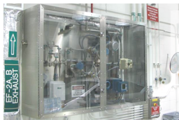
FTIR Emissions Analyzer for non-Regulated Emissions
