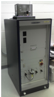
FTIR Emissions Analyzer for non-Regulated Emissions
