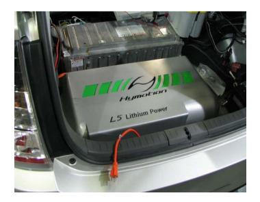
5 kWh Li-ion battery system installed in parallel to the production battery
