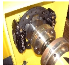
Figure 26: Disc brake and its actuator to simulate the driver commands
