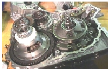
Figure 18: Removal of the CVT oil pump
