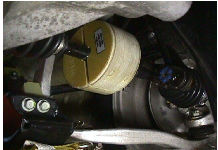
Figure 5: Half-Shaft Honda Insight Torque Sensor
