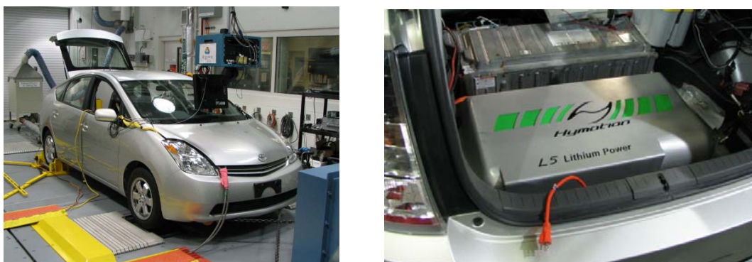
Figure 16: Hymotion PHEV Prius on Chassis Dynamometer with Hymotion 5-kWh Battery System Installed in Parallel to the Production Battery
