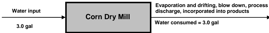
FIGURE 20 Water Input and Consumption of an Average Corn Dry Mill Producing One Gallon of Fuel Ethanol (RFA 2007)
