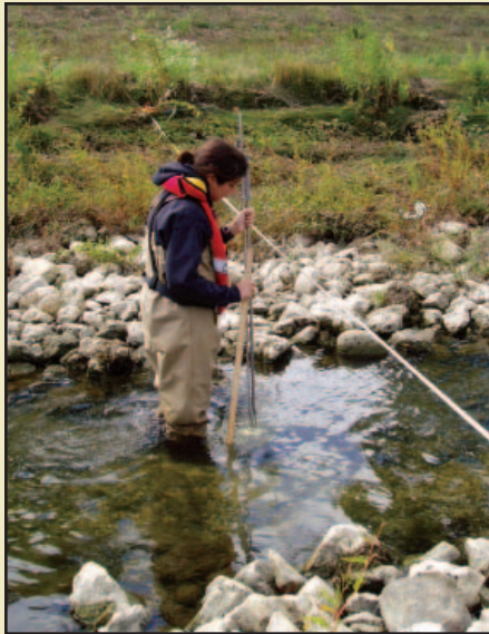
U.S. Geological Survey personnel collecting streamflow measurements.
