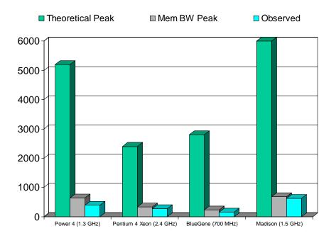
**Fig. 3.** Memory bandwidth bound for sparse matrix-vector product. Only one vector (N=1) is considered here. The matrix size has  $\mathtt{m}=90{,}708$  rows and  $\mathtt{nz}=5{,}047{,}120$  nonzero entries. The processors are 1.3 GHz IBM Power 4, 2.4 GHz Intel Xeon, 700 MHz IBM BlueGene, and 1.5 GHz Intel Madison. The memory bandwidth values are measured using the STREAM benchmark.
