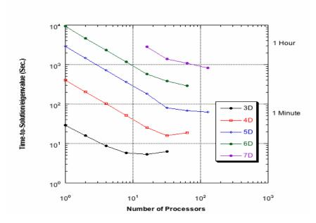
**Fig. 1.** Sample parallel performance of the CRP code on up to 128 processor of IBM SP3 at NERSC.
