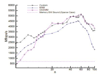
**Fig. 4.** Performance of the tensor matrix vector multiplication for three dimensions on Intel Madison (1.5 GHz) processor. The custom code is manually optimized code, MXM code is from [12] and DGEMM() routine is from Intel's MKL library. Note that the sparse matrix vector multiplication will only do at most about 687 Mflops/s based on the memory bandwidth bound on this processor.
