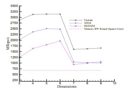
Fig. 5. Performance of the tensor matrix vector multiplication for n=7 in all dimensions. The sharp drop in performance is due to the working set of the problem going out of the L2 cache (4 MB) of the Intel Madison processor. We are trying to contain this drop (to some extent) with better implementation (with extra blocking). Notice that the DGEMM() does not perform well for small values of matrix sizes and especially when the two matrix sizes are vastly different (large dimension case).
