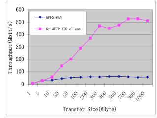
Figure 4: Comparison of performance of the XIO client with GPFS WAN mounted at Argonne
