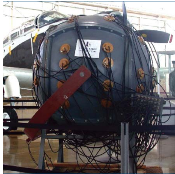
Atomic Weapon Using Triggered Spark Gaps
