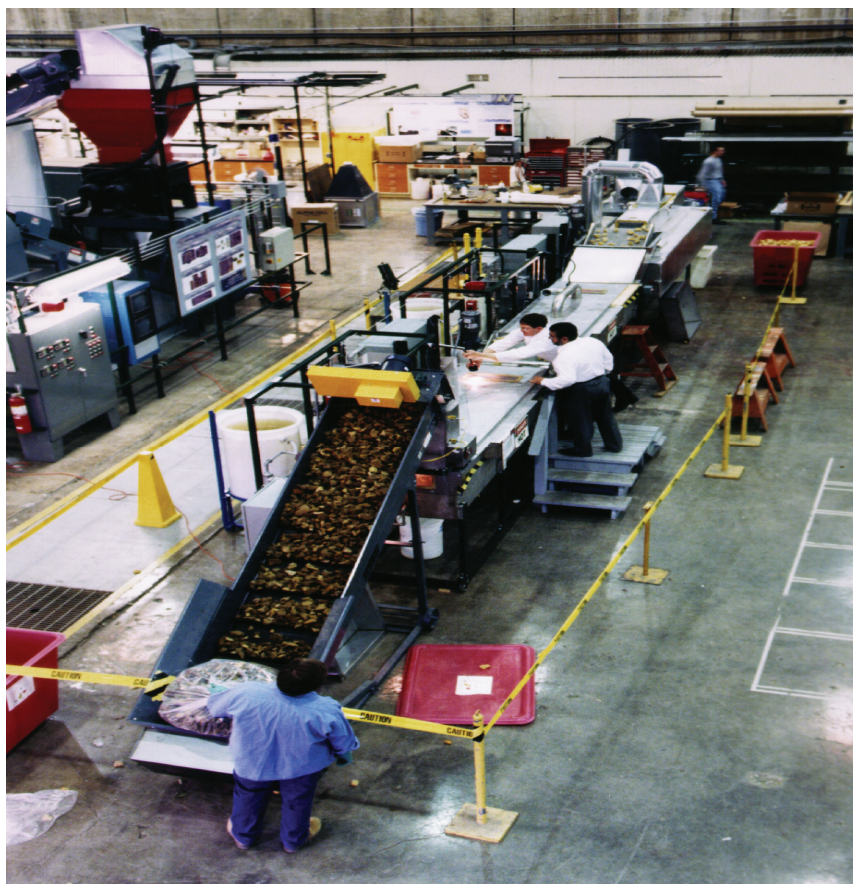
FIGURE 8.2 Wash, Rinse, and Dry Continuous Equipment
