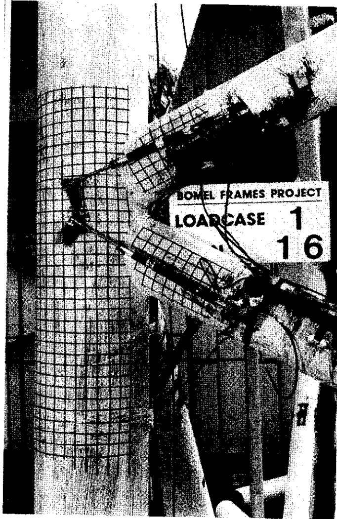
Figure 2.9 Distortion of the Node 38 chord around the compression intersection (upper)
