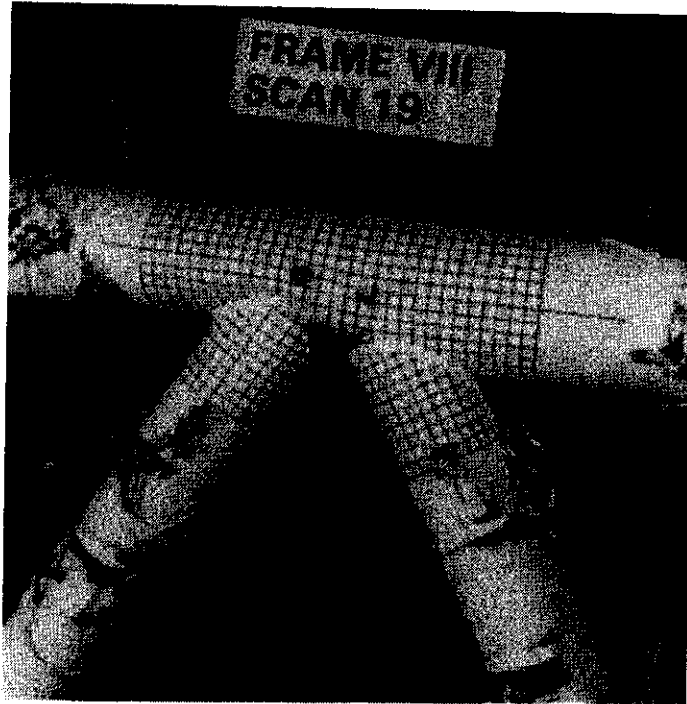
Figure 2.20 Phase II - plane frame test \beta = 0.77 K joint distortion - Frame VIII Scan 19
