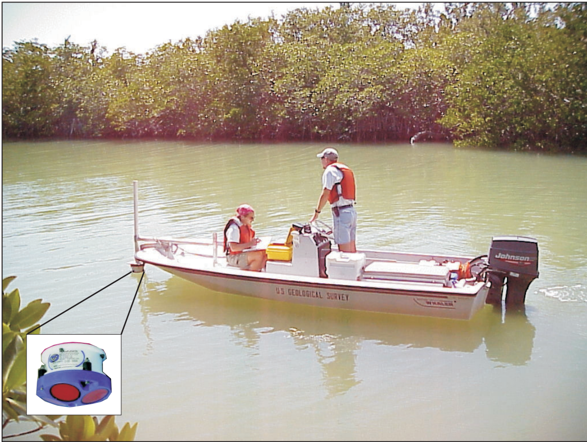
Figure 7. Boat-mounted Acoustic Doppler Current Profiler for measuring discharge at the Trout Creek monitoring station. Doppler is shown in inset.
