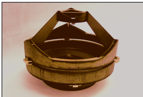
▲ This photograph shows part of the structure of a telescope that San Diego Composites, Inc., has been developing with its carbon-carbon material, an alternative to toxic beryllium.
