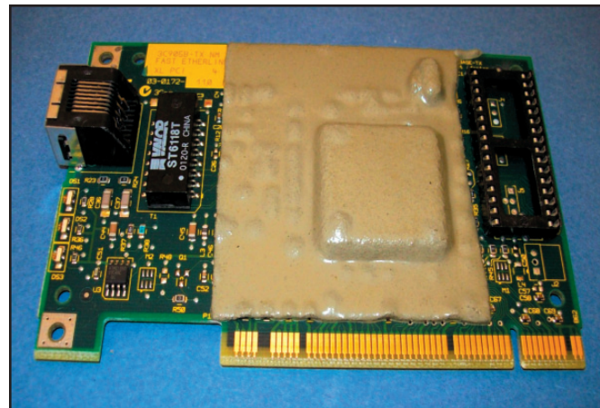
▲ Cornerstone's material minimizes vibrations that can damage components of circuit boards and other electronic devices.
