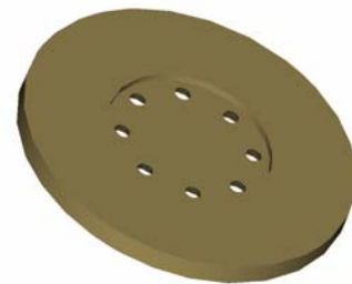
Figure 2. Schematic of a basic 8-hole turbulence nozzle configuration.
