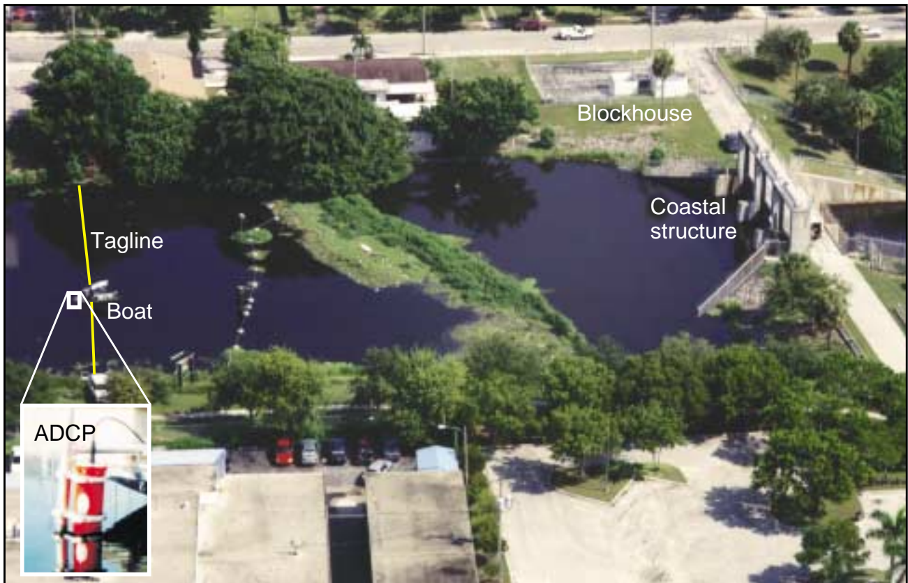
Figure 5. Typical field setup for an Acoustic Doppler Current Profiler (ADCP) measurement of streamflow for structure S-15 on the C-51 canal.
