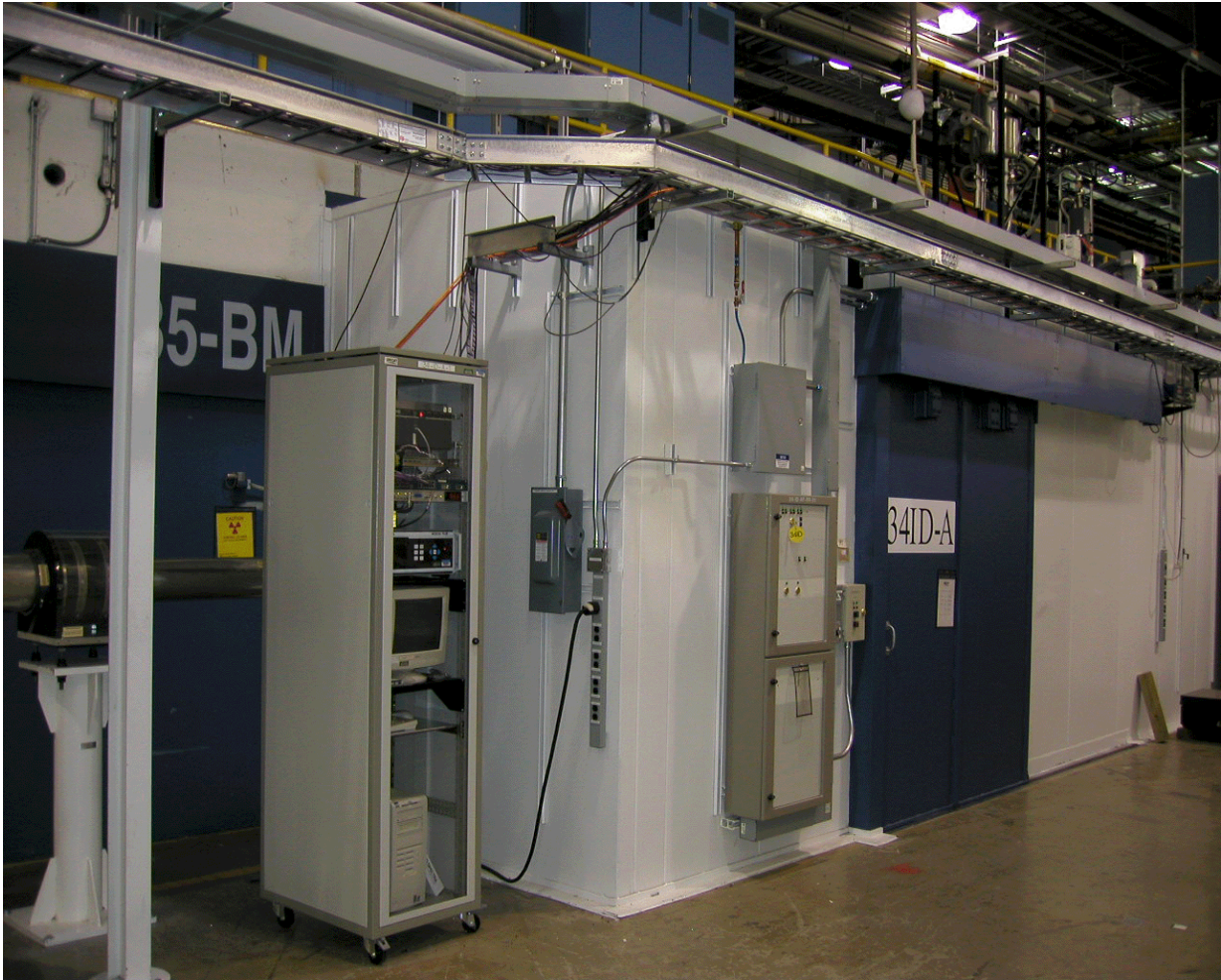
Figure 3.31 Typical First Optics Enclosure
