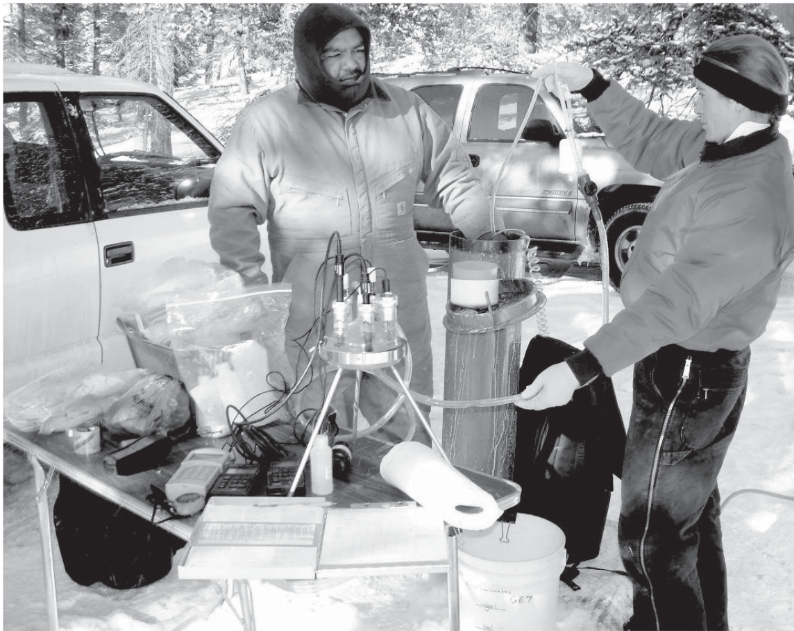
Figure 7. Sampling equipment, including flow-through cell and water-quality-parameter measurement instruments.
