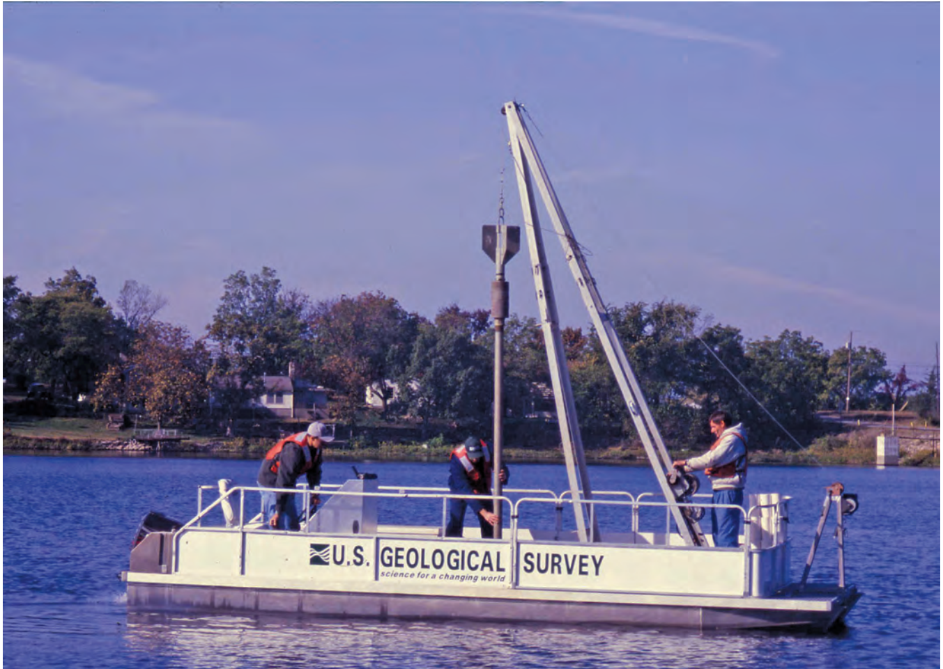
Figure 2. Photograph showing pontoon boat mounted with gravity corer used to collect bottom sediment cores from Shawnee Mission Lake May and November 2006.
