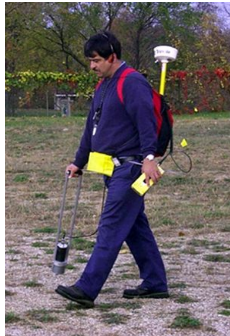
Use of a gross gamma screen and global positioning system provides real-time data for an adaptive sampling and analysis program.
