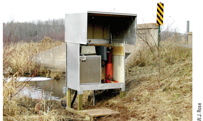
Figure 7. Typical U.S. Geological Survey recording streamflow-gaging station with automatic water sampler for load determinations.
