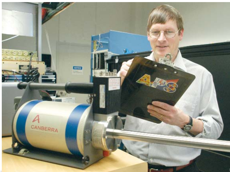
Fig. 1. Steve Ross (AOD-TBS) with a germanium energy dispersive detector, one of several detector types that users can check out from the APS Detector Pool.
