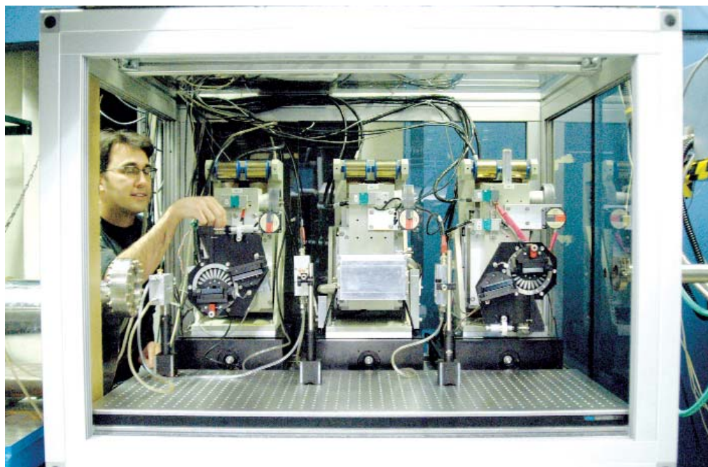
Fig. 1. XOR staff member Tom Toellner at the new monochromator used for HRIXS. The cryogenically-cooled, high-resolution monochromator transmits a 1.2 meV-bandwidth x-ray beam with 60% spectral efficiency.
