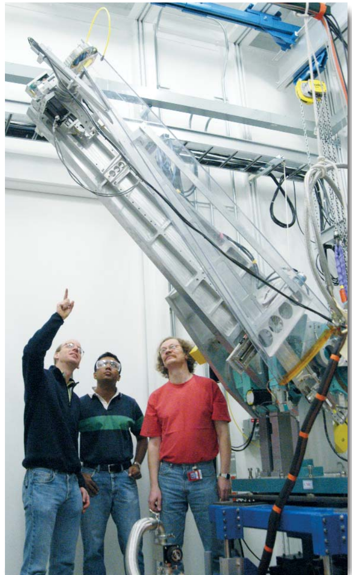
Fig. 1. John Hill (BNL), Nalaka Kodituwakku (Western Michigan University) and Thomas Gog (CMC-CAT) inspect the spherical analyzer on the detector arm of the new IXS spectrometer in sector 9.
