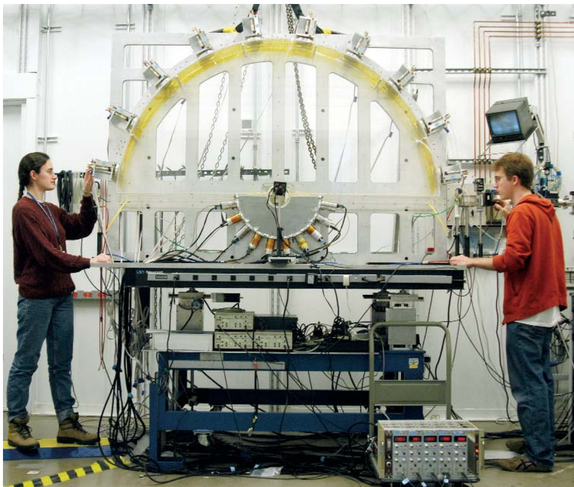
Fig. 1. University of Washington graduate students Adrienne Battle (left) Tim Fister inspect the alignment on the q IXS apparatus at sector 20-ID (PNC-CAT). This apparatus, which will soon become available to general users, is primarily used to measure the contribution to the dynamical structure factor from the core shells of low-Z elements or weakly-bound orbitals of higher-Z elements. This provides an alternative to and extension of x-ray absorption spectroscopy measurements performed with soft x-rays.
