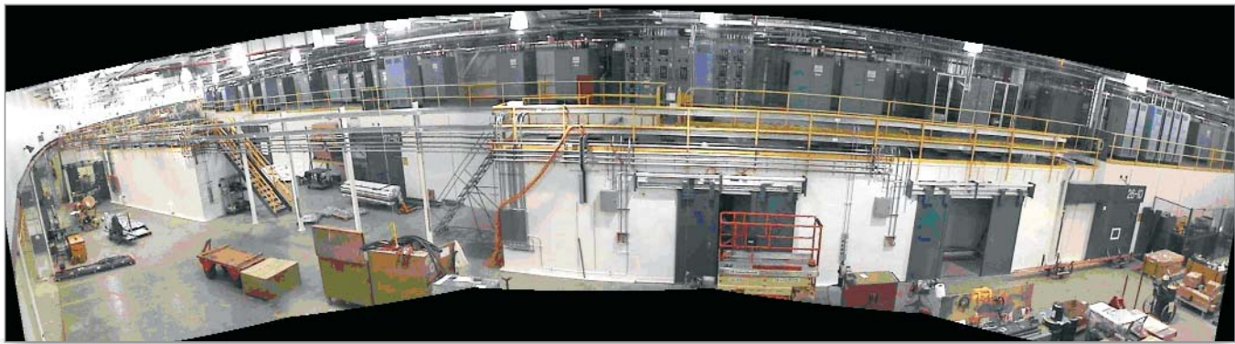
Fig. 2. The Nanoprobe beamline at APS sector 26 as of late 2004, with hutch construction complete. The first optical enclosure is in the center of the photo; the second optical enclosure and the Nanoprobe end station are at left. (Photo: R. Winarki, XFD-XMG)
