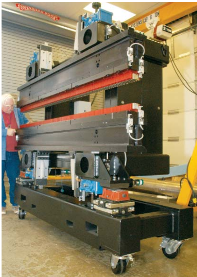
Mike Merritt (XFD-XFE) with one of the new planar hybrid IDs (period length 2.7 cm) after testing and just prior to installation.
