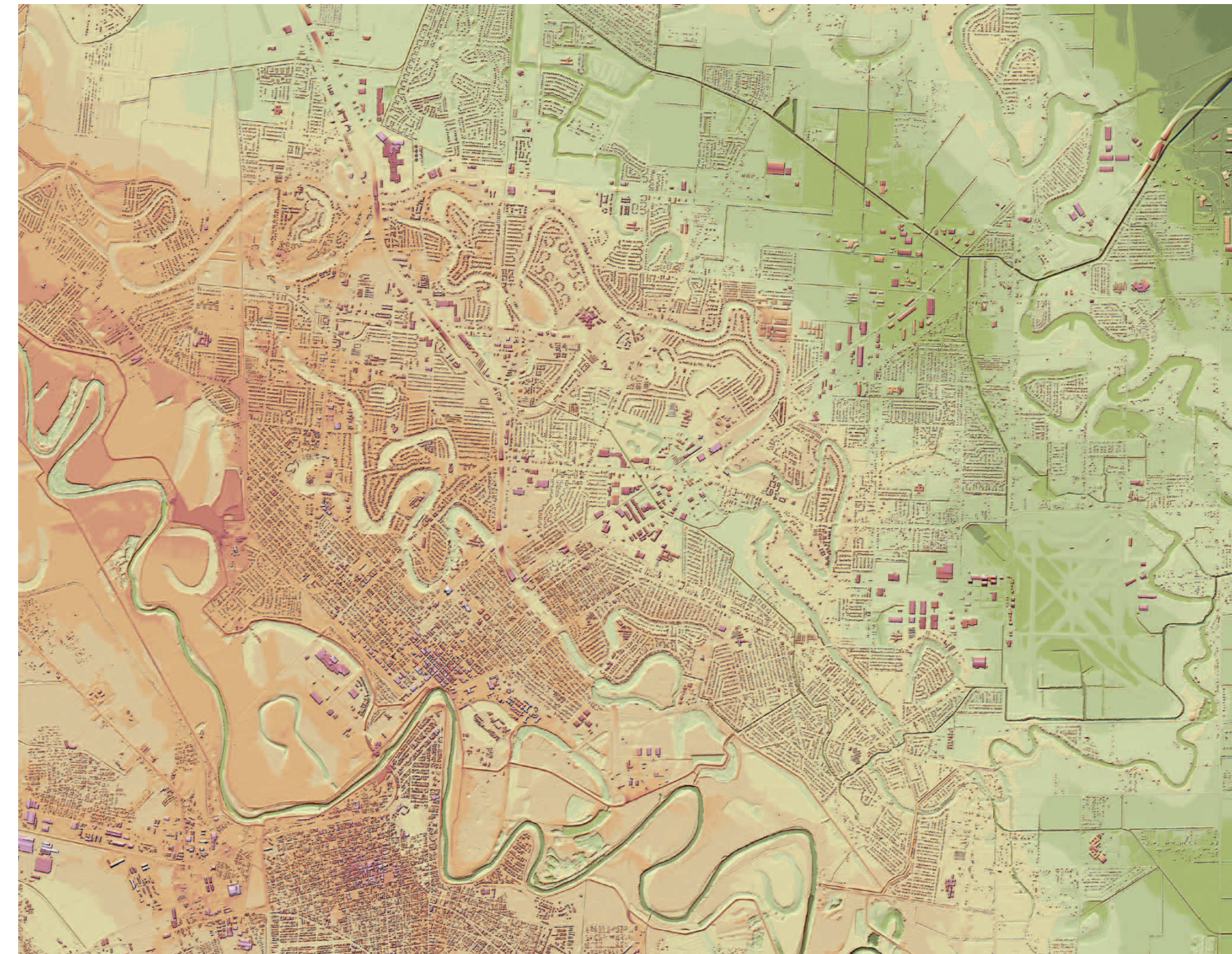
Digital terrain model created using LIDAR data in Brownsville, which will be integrated into the seamless National Elevation Dataset layer of The National Map .
