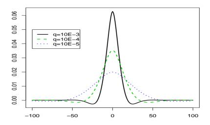
Figure 3: Low-Pass and Band-Pass Gain Functions ( $m=1,q_{\zeta}=.25,q_{\kappa}=4$ )
