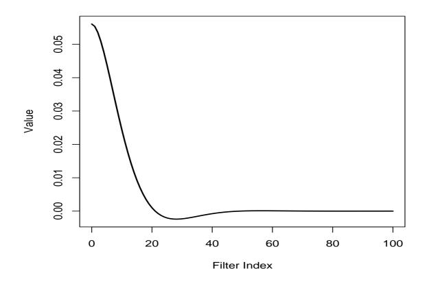
Figure 2: Exact weight coefficients for the HP filter.
