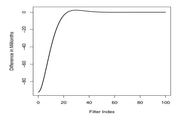
Figure 3: Difference of weights  $\varphi_j - w_j$  for the HP filter. Vertical scale is in millionths.
