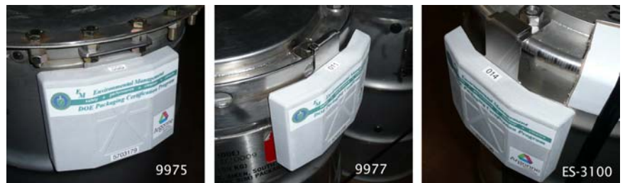
RFID tags mounted on Models 9975, 9977 and ES-3100 drums
