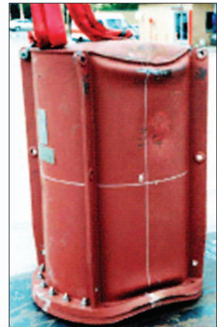
SAFESHIELD 2999A packaging after drop test
