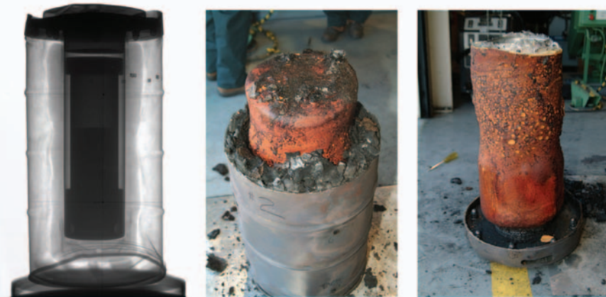
Digital radiograph showing silhouette of intact primary containment vessel (left), charred outer and intact inner polyurethane foam (center), and intact polyurethane foam (right)
