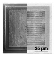
The figure above shows two views of the same area of interest in a 10-micrometer-thick semiconductor bond pad. At left is a conventional SEM image. At right is an SCEM image of the same area, showing details of the internal microstructure that are hidden from view in the SEM image.
