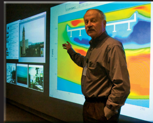
Engineer Ron Kulak stands in front of a visualization of water flowing around bridge supports. The redder colors represent faster flow rates. High-performance computing provides engineers with the ability to visualize the flow in unique detail.
