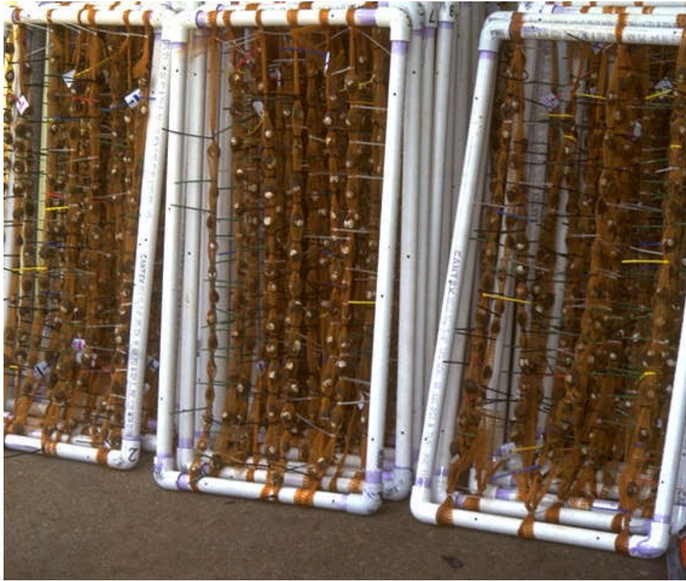
5. PVC cages containing clams prior to deployment
