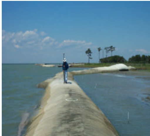
Figure 7a and 7b. RTK Base Station and Using Rover GPS on Geotubes
