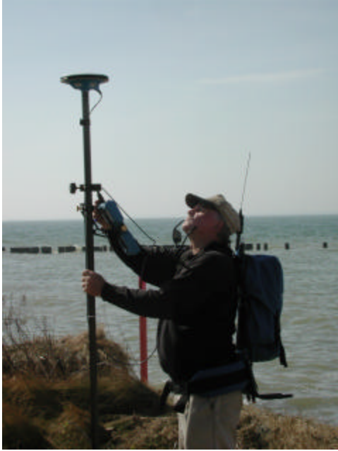
Figure 7. Kinematic GPS showing the roving receiver collecting data at various points of interest such as land/water interface, abrupt vegetation change, and geologic features.
