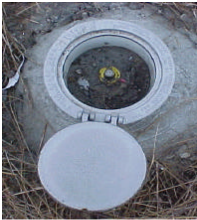
Figure 6. Tidal benchmark with capped PVC flange denoted as 8571579 A TIDAL.
