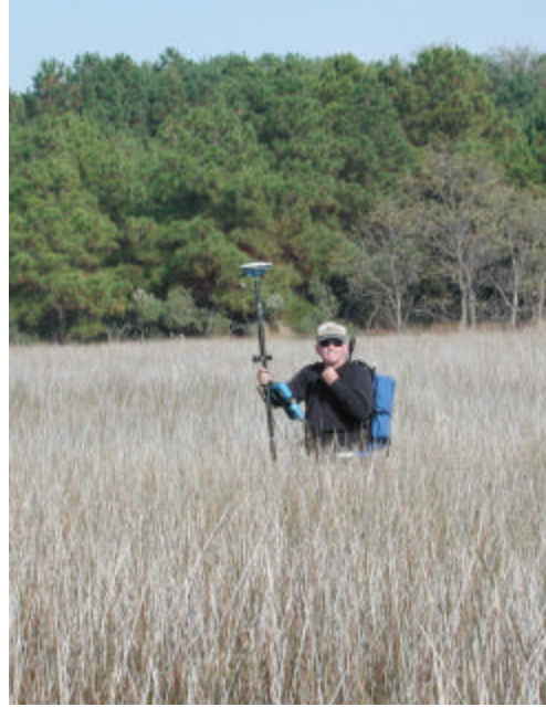
Figure 7. Kinematic GPS showing the roving receiver collecting data at various points of interest such as land/water interface, abrupt vegetation change, and geologic features.
