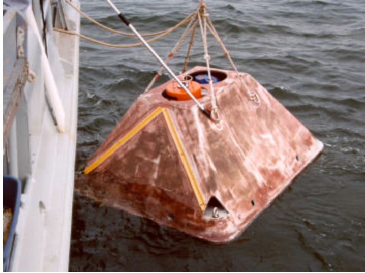
Figure 4. The bottom mounted ADCP transducer head (in blue) can be seen as it is lowered to the Chesapeake Bay floor for waves and current data collection.
