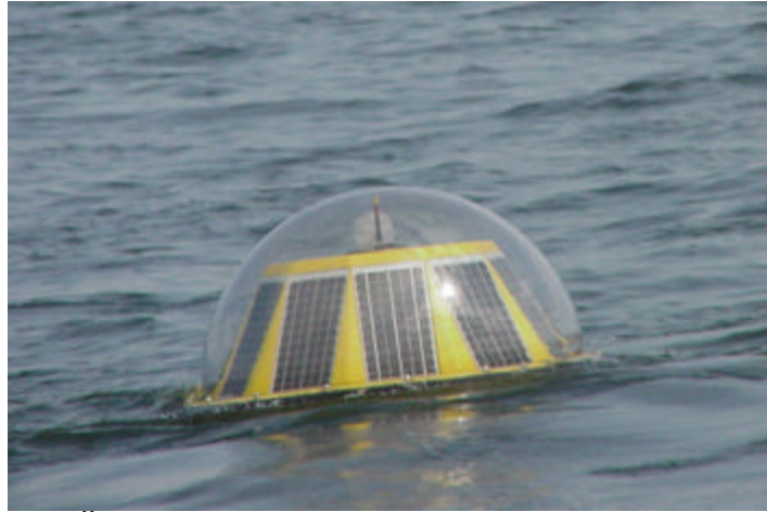
Figure 3. TriAxys ® Wave Buoy collecting data in waters around Barren Island.
