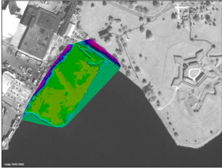
Figure 5. The Ft. McHenry Pre-construction Digital Elevation Model (DEM)
