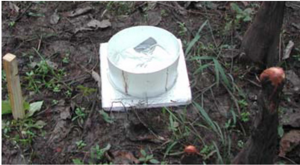
Figure 5. Litterfall collector for the production study (latitudinal test of the curvilinear model). The collectors float on the water. The foil inside of the trap is covered with Tanglefoot® (flypaper glue) so that leaves, twigs, and seeds that fall on the trap are captured (Middleton, 1995).
