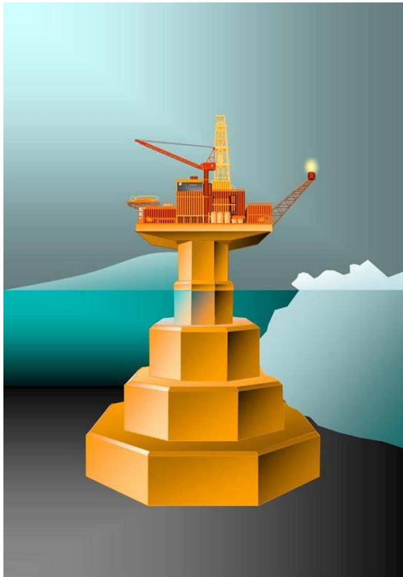
Figure 3-11: Steel Stepped Gravity Base Structure
