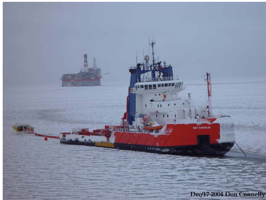
Figure 3-30: “Smit Sakhalin” Connected up to SALM Production Buoy Preparing for Winter Lay Down Operations (Courtesy of DC Marine)
