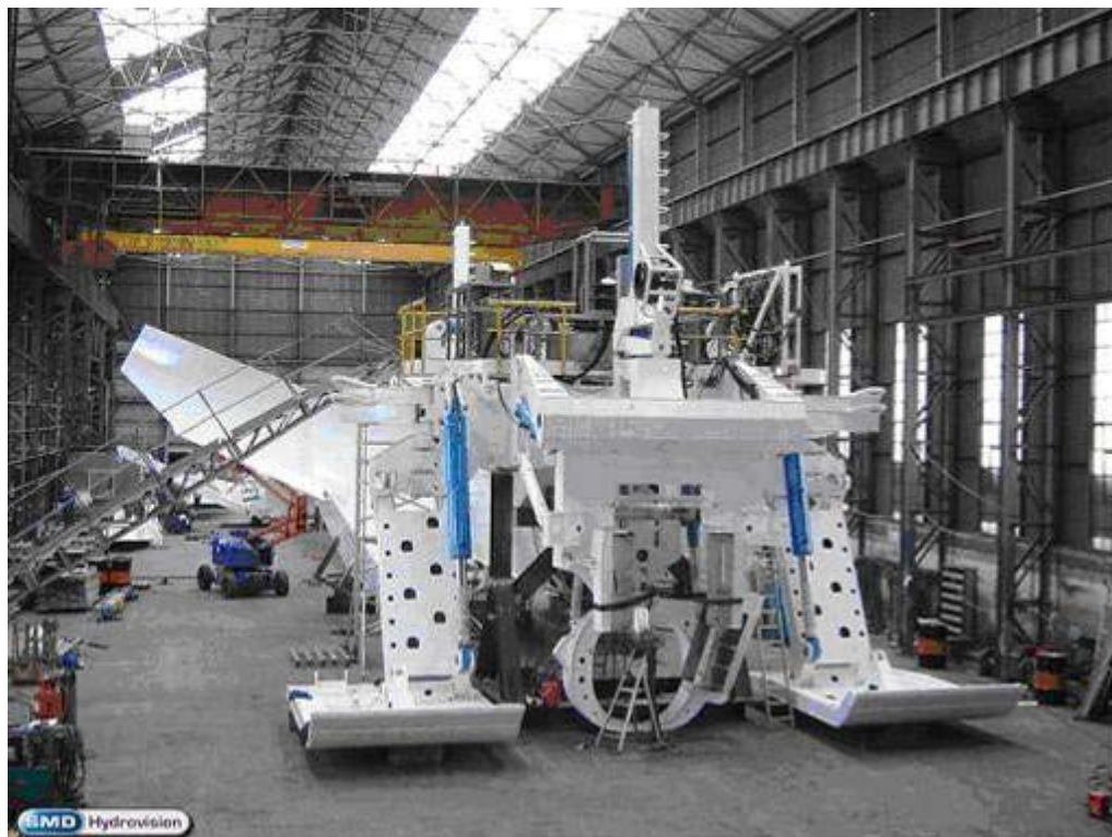
Figure 4-35: Typical Subsea Plow (Courtesy of SMD Hydrovision, 2007)
