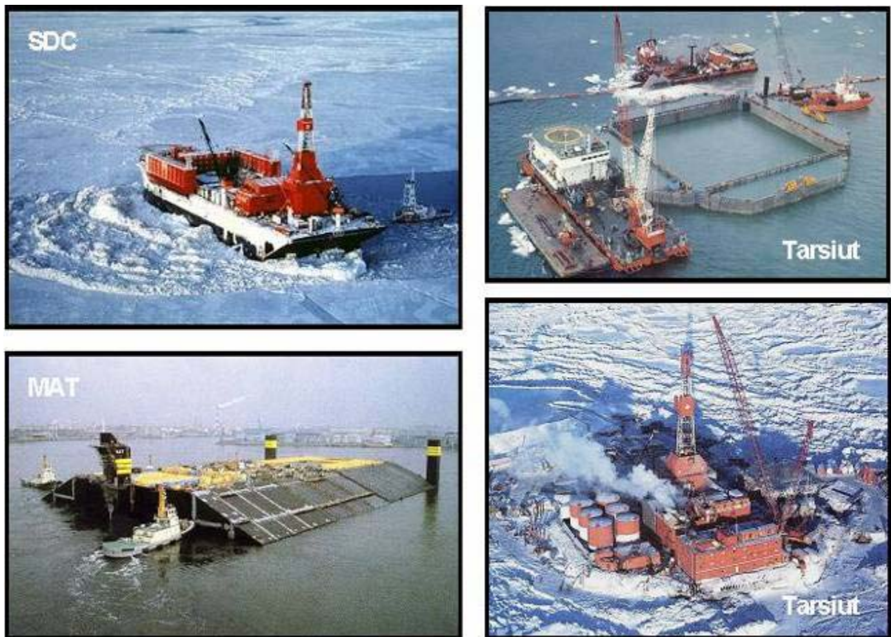
Figure 2-1: Arctic Caisson Drilling Structures
