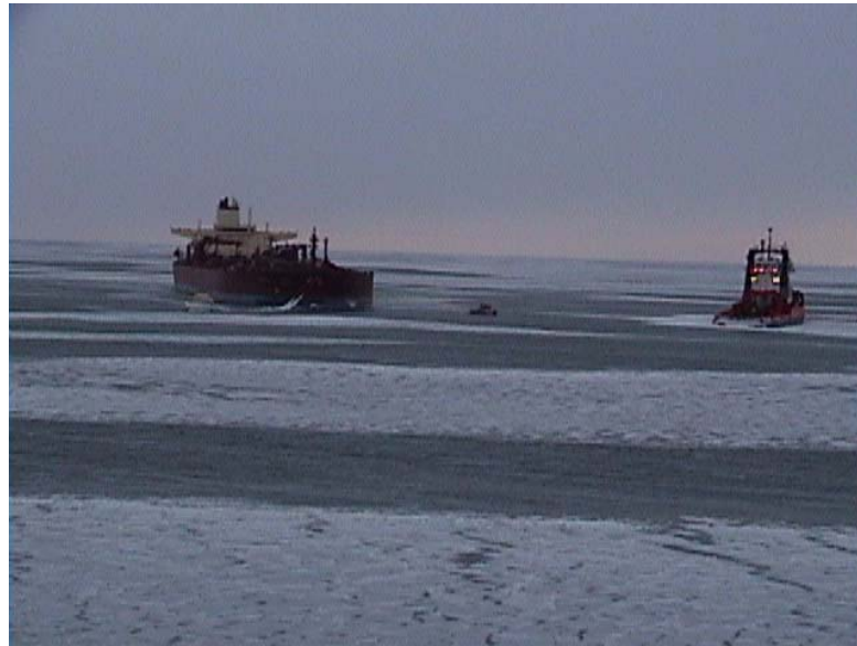
Figure 3-32: FSO “Okha” Connected up to Production SALM Buoy, Late Season (Courtesy of DC Marine)
