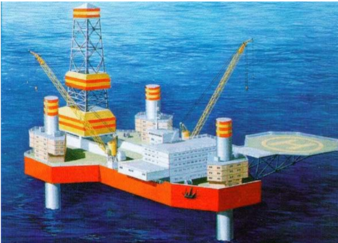
Figure 3-15: Ice Resistant Jack-up Arkticheskaya 6500 / 10-30 (JSC Gazprom, 2007b)
