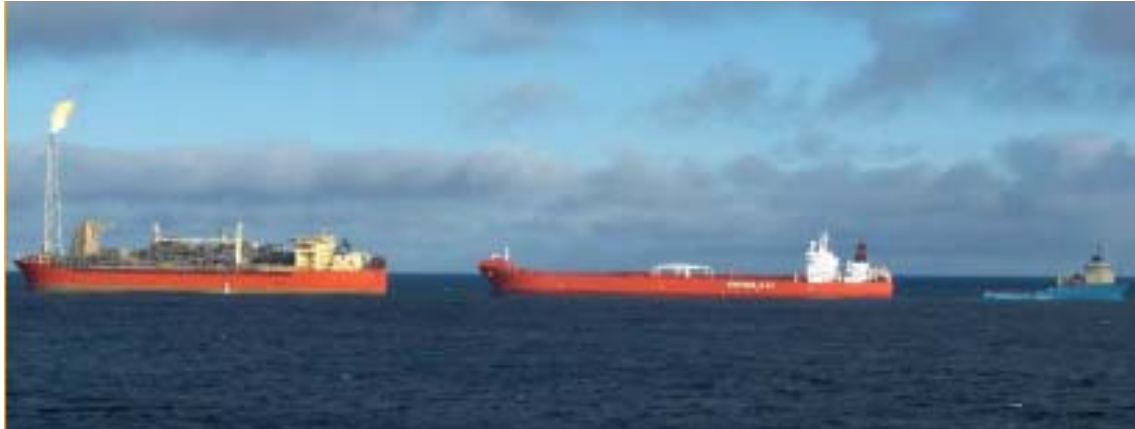
Figure 3-24: SeaRose Offloading to Shuttle Tanker (Howell, 2007)
